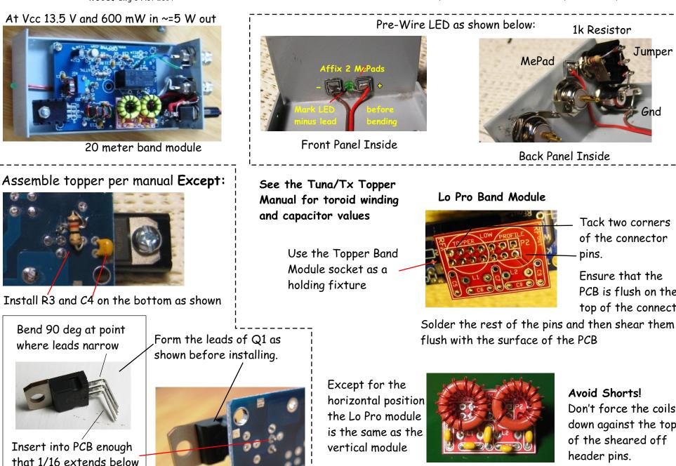
Avoid Shorts! Don't force the coils down against the tops of the sheared off header pins.
